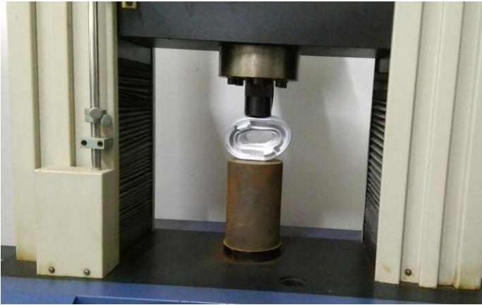
No crack on forging surface when compressed by testing machine
